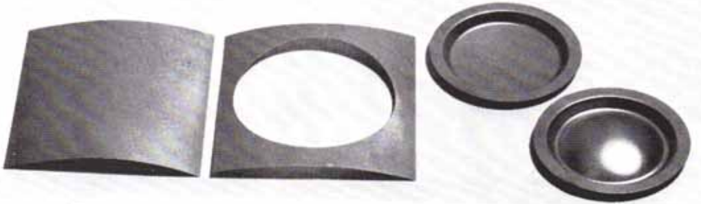
Figure 1: Steps in transforming a piece of metal into a rupture disk.
